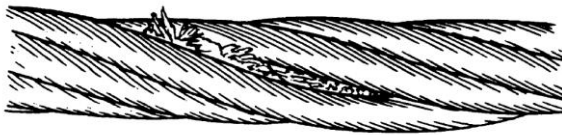
Figure: Local rope diameter increase
