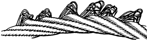
Figure: Example of wire displacement
